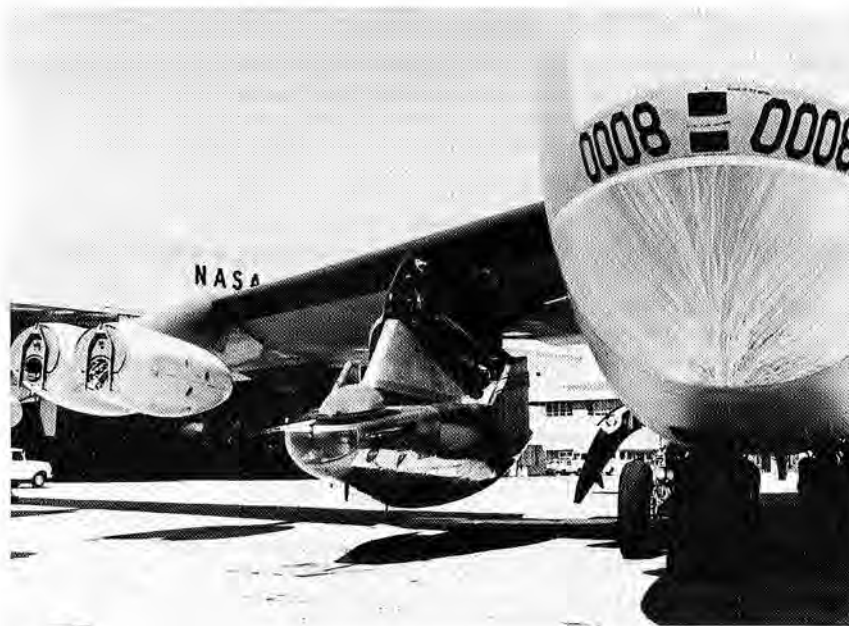
October 12: M2-F2 lifting body mated to B-52 launch aircraft at NASA Flight Research Center, in preparation for flight tests.
